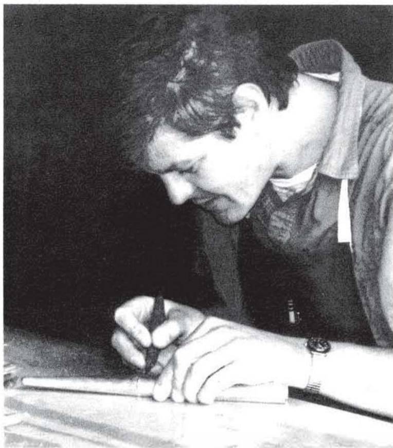
Martin Pasi cutting the mouth in a small pipe—a very delicate process.
