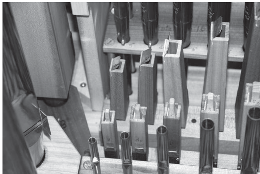
Small Positive wooden pipes of the Flöte douce 8 and Hohlflöte 8
