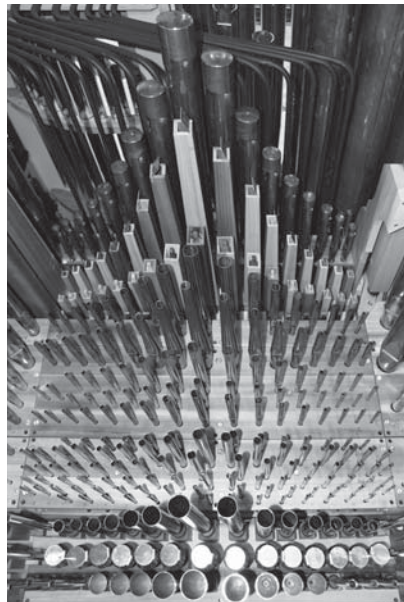
Positive treble pipework with façade tubing in background
