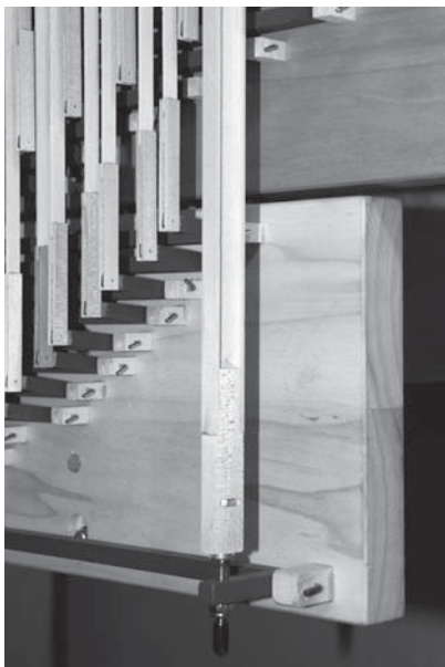
Key action with compensator system for humidity changes
