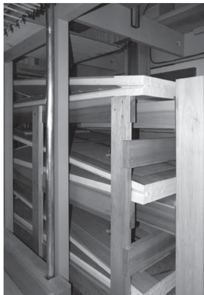
Bellows stack located in the rear of the organ base
