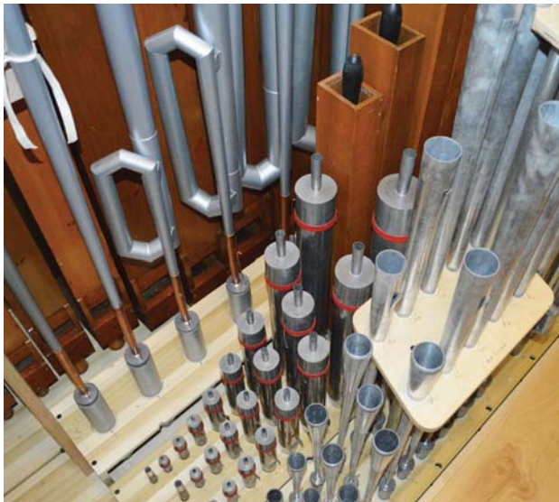
Swell unit stops including 16-8-4 Fagott (photo credit: Parsons Pipe Organ Builders)
