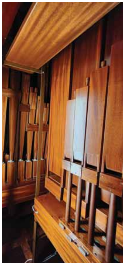
Pedal Soubasse and Bombarde pipes with walkboard, all made of mahogany
