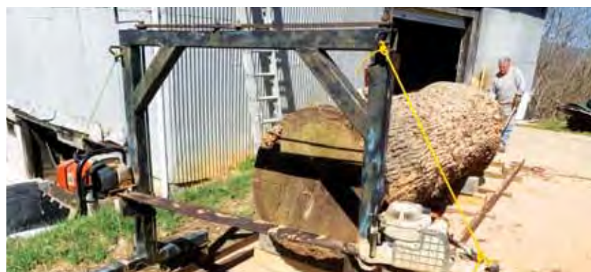
Splitting an oak log on the bandsaw at the sawmill of Taylor & Boody (photo credit: John Boody)
