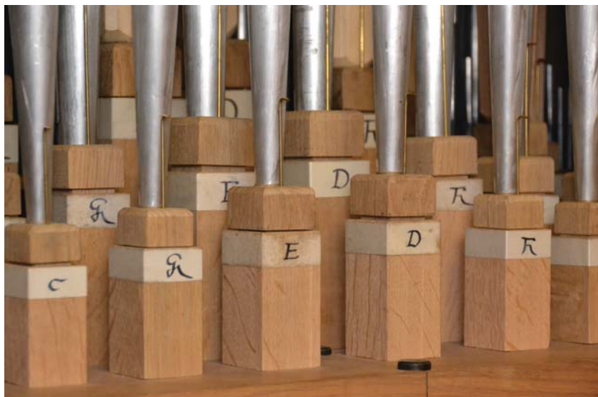
Reed boots mortised into the toeboards. The tops of the boots have a strip of parchment wrapped around them for reinforcement
