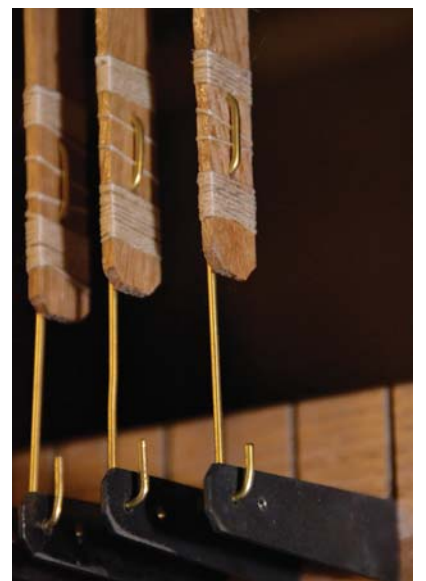
Detail view of tracker ends with hand-bent brass wires hooked into the squares
