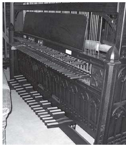
Retaining original frame but reworking worn keys, pedals and action, new clavier now has world-standard layout, making it easier for guest carillonneurs (photo credit: Wylie Crawford)
