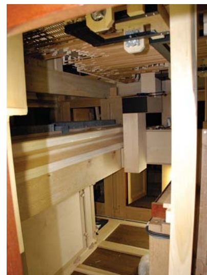
Interior of the organ showing bellows and Great key action
