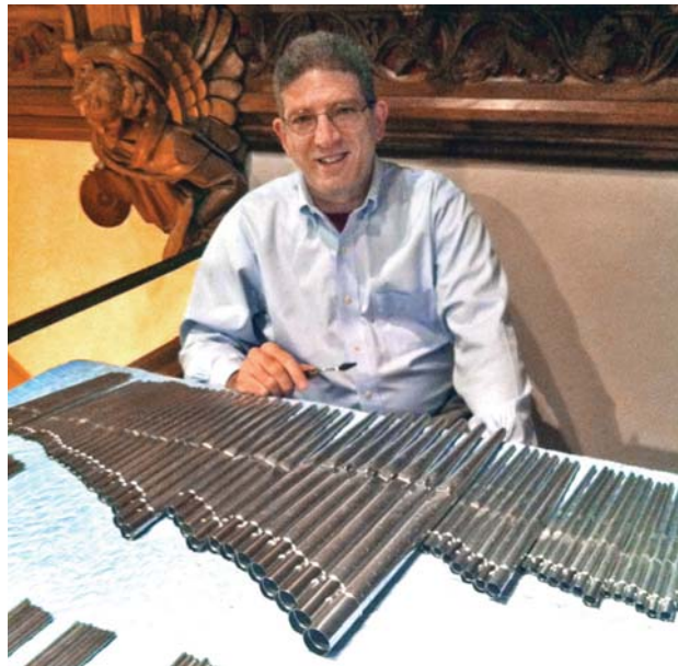
Sebastian M. Glück in the organ loft with the voiced pipes of the Mixture, ready for installation and tonal finishing
