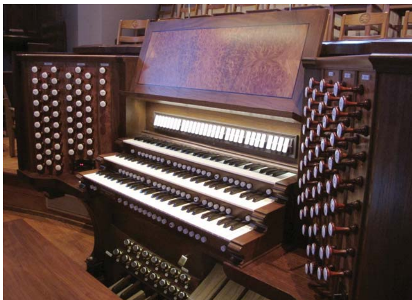
The organ console, with a case of quarter-sawn white oak and walnut interior, enriched with Carpathian elm burl (photo by Lynn Dobson)
