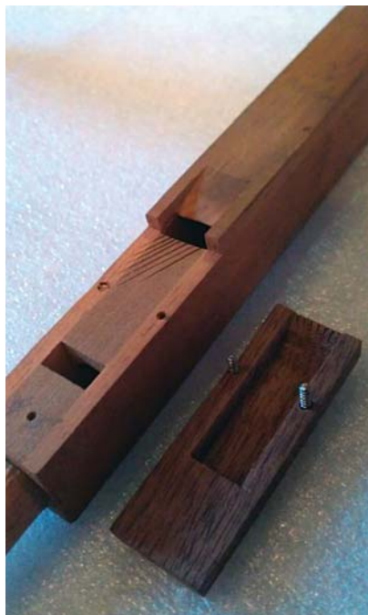
Voicing details of the Flauto Traverso 4'
