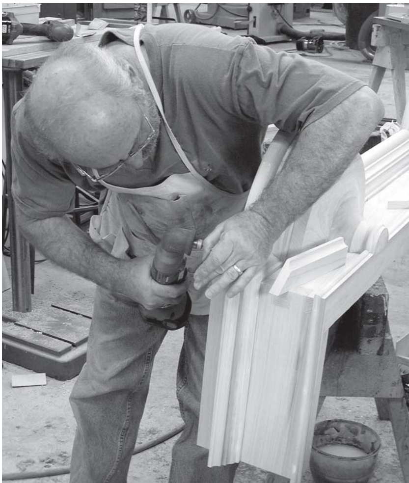
Craftsman Dale Krause applying moldings to the casework impost
