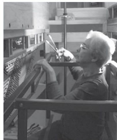
Church member Betsy Oerter adjusting Haskell bass pipes of the Diapason and Flûte Traversière in the Swell windchest
