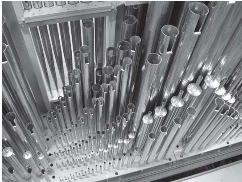
Treble pipework from the façade to the back of the Great slider windchest
