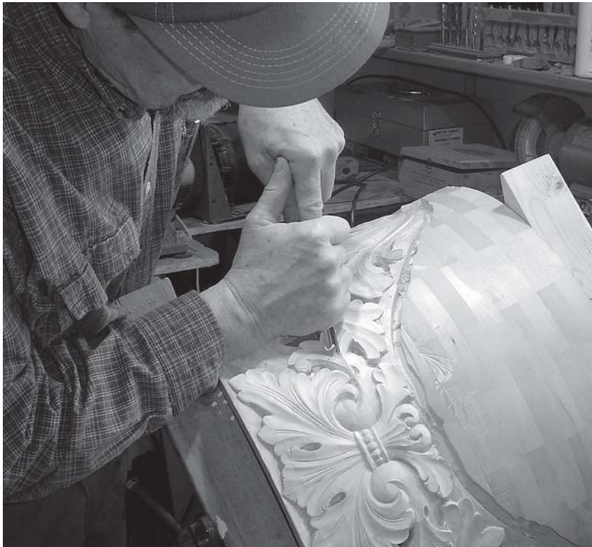
The skilled hands of traditional woodcarver Arnie Bortnem fashioning the pipe shades from basswood carving blanks for the Kernersville Chapel organ
