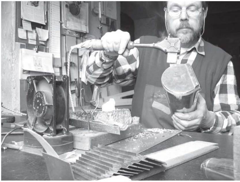
Pipemaker Toni Kaes soldering the languid to the foot of one of the façade pipes
