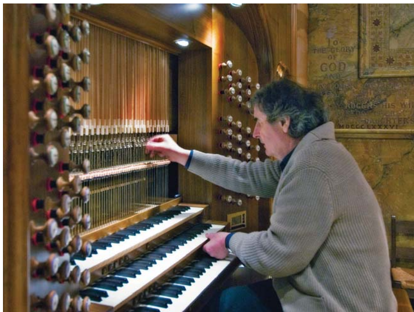
Pascal Quoirin adjusts the trackers of the mechanical console
