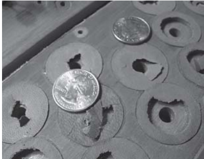
Photo 8, spool-box contact pouches before
