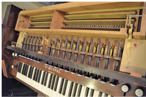
Figure 3. Interior of 1903 Mustel Art Harmonium, showing multiple sets of brass reeds
