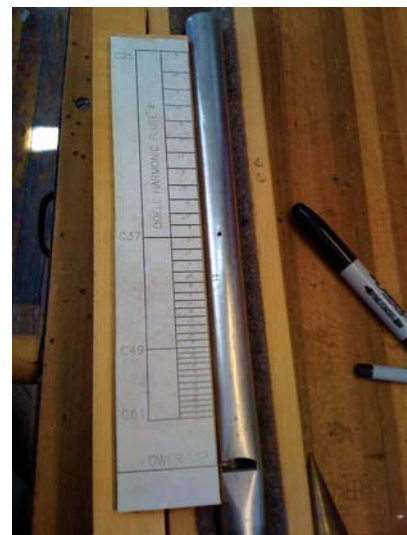
Comparing nodal points on the Harmonic Flute 4' with scale data from Odell Op. 178
