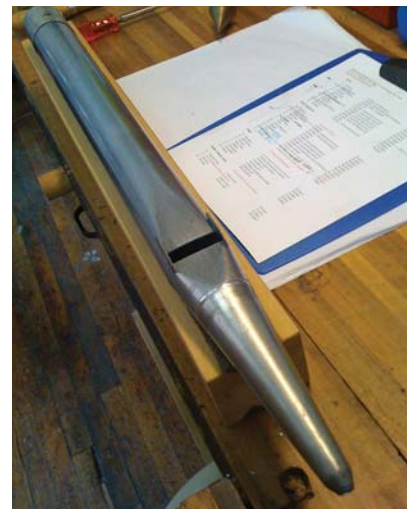
Repaired pipe foot for one of the notes of the Great Open Diapason 8'. Note the use of common metal and the 2/7 mouth.
