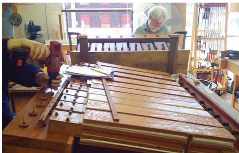
Rebuilding pneumatic stop-action assemblies
