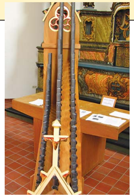
The Rims organ: two 8’ ranks and one 6’ rank all with the same (27mm, “pigeon’s egg”) diameter (photo: Jos van der Giessen)
