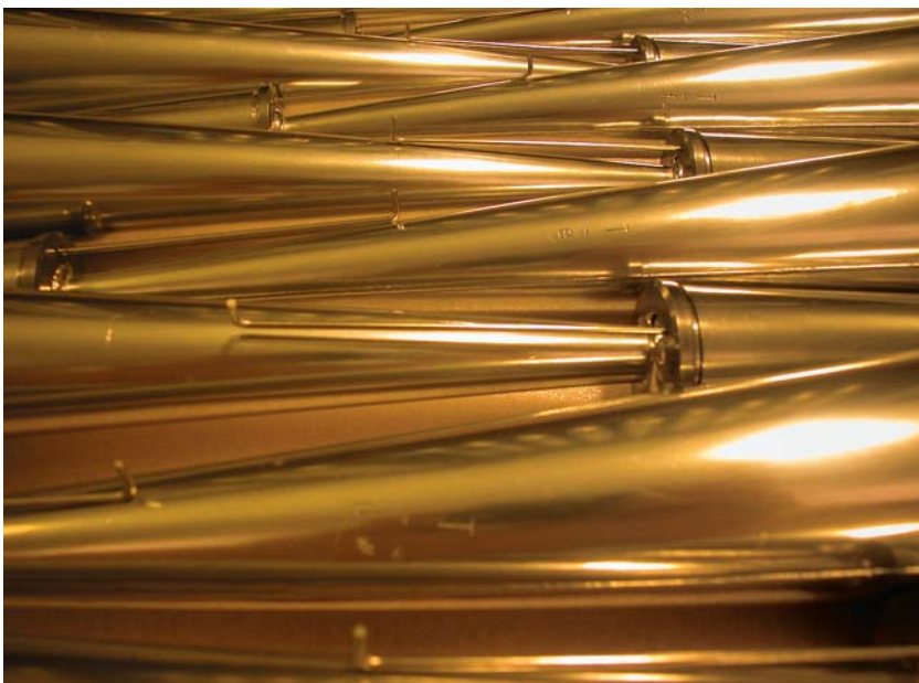
New trumpet resonators ready for installation
