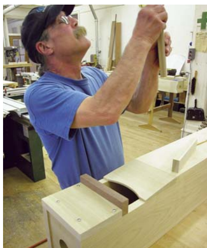
Constructing new wood pipes in the shop
