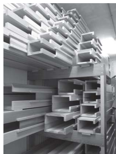
Violone and Open Wood pipes stacked in position on the roof of the organ (photo credit: Louis Patterson)
