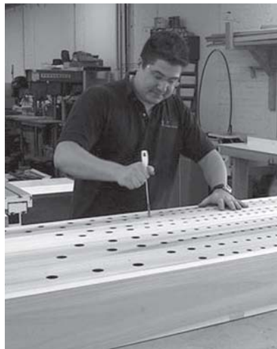
Shop foreman John Williams brushing toe holes in one of four new manual windchests
