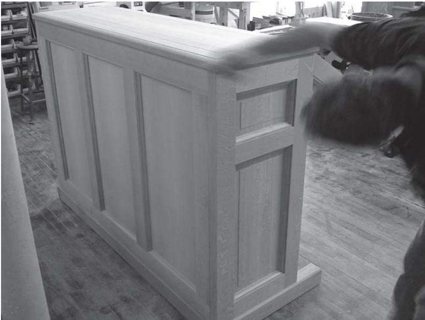
Curt Goettlich sanding the new console carcass
