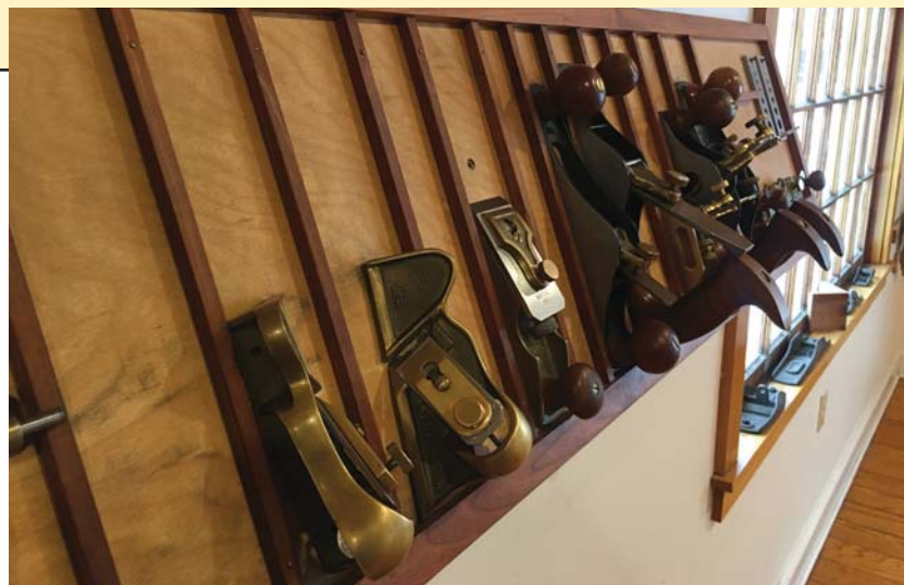
In the foreground, "left and right" versions of Lie-Nielsen's reproduction of the Stanley #95 Edge Plane
