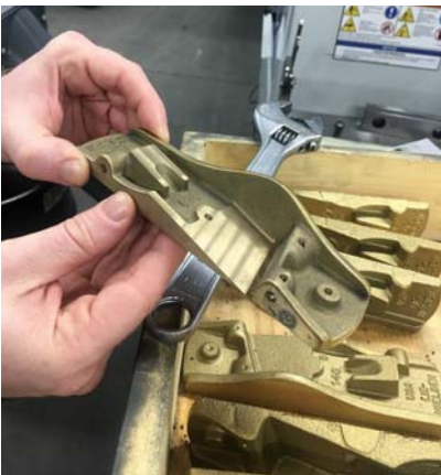
Bronze casting, halfway through the process
