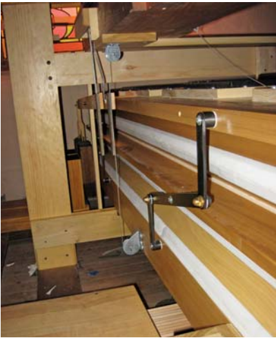
2. Double-rise reservoir (Photo credit: Nicholas Ringwald)
