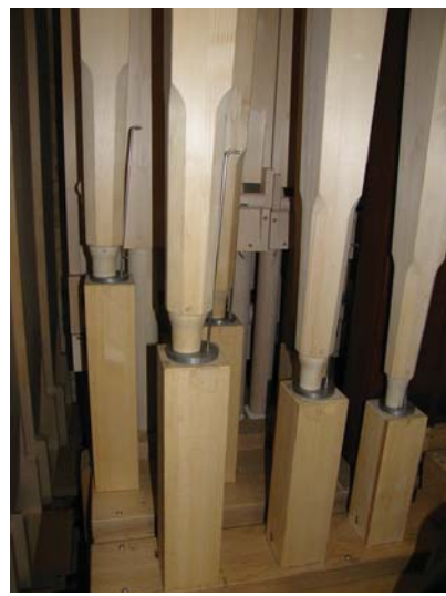
32' Contre-Bombarde wood pipes
