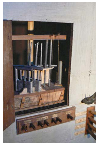
Figure 3. The bird stops of the Bonatti organ in Verona
