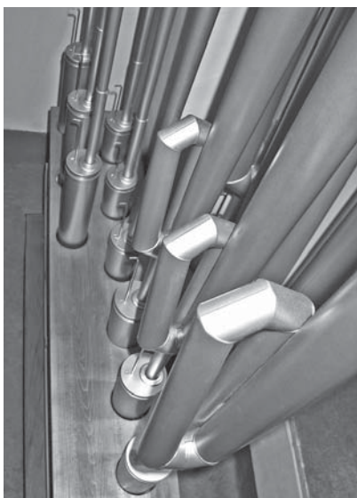
The bottom octave of the new full-length 16' Basson; CCC, CCC#, and DDD stand behind. (photo credit: Sebastian M. Glück)
