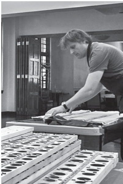
Robert Rast preparing internal windchest components for releathering (photo credit: Sebastian M. Glück)
