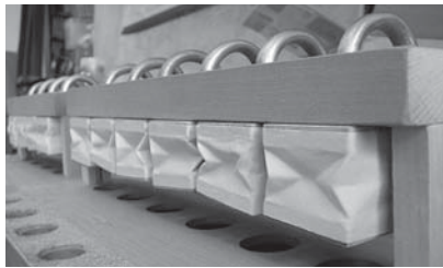
Releathered box pneumatics prior to valve replacement (photo credit: Robert Rast)
