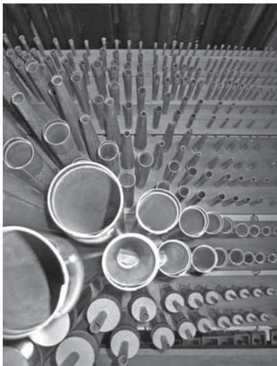
The upper Great windchest, with the façade pipes at the top, and the new 16' Subbass on the lower level (photo credit: Sebastian M. Glück)
