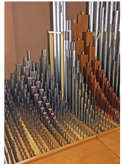
One side of the two slider soundboards for the Choir fluework (photo credit: Sebastian M. Glück)
