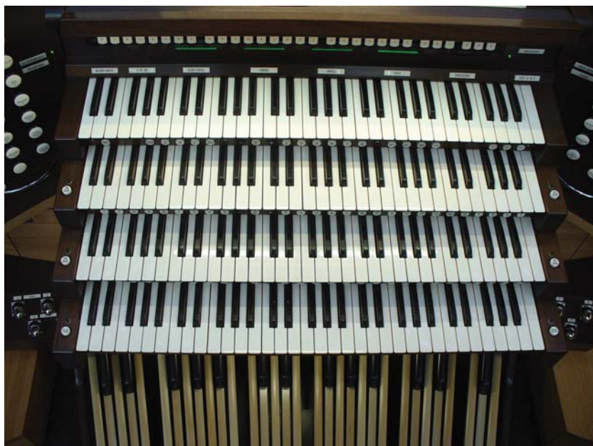
The console's four manuals have bone overlays for the natural keys, with the accidentals in solid ebony. The pedalboard notes are made from maple, with ebony caps for the accidentals.
