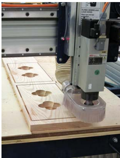
Case details being machined on the CNC router
