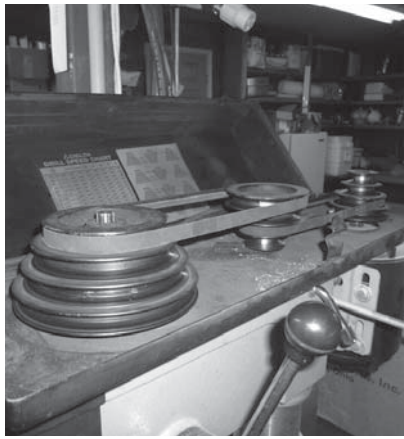
Drill-press pulleys set on almost highest speed
