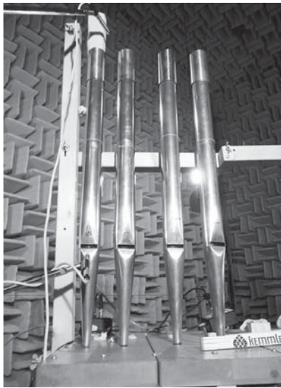
The "mouth tone" of a pipe is being recorded. Sound-absorbent material is inserted inside the pipe body to prevent the development of the sound column.
