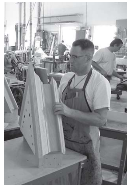
Woodworker Jon Taylor finishes capitals
