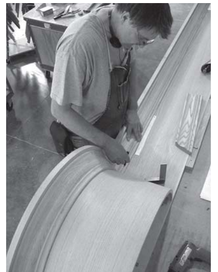
Woodworker Ed Stibal fits molding to the impost
