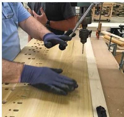
Completing final borings for windchest primary boards
