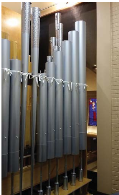
The 16' Bombarde with Haskell construction, where the pipe is inverted on itself. This is a full-length speaking pipe in half the height.
