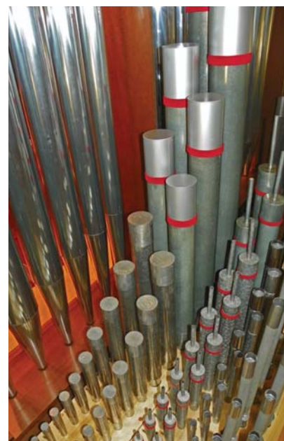
A view into the Positiv behind the speaking façade pipes: 8' Bourdon, 4' Rohrflöte, 2' Recorder, and 8' Clarinet (photo: Sebastian M. Glück)
