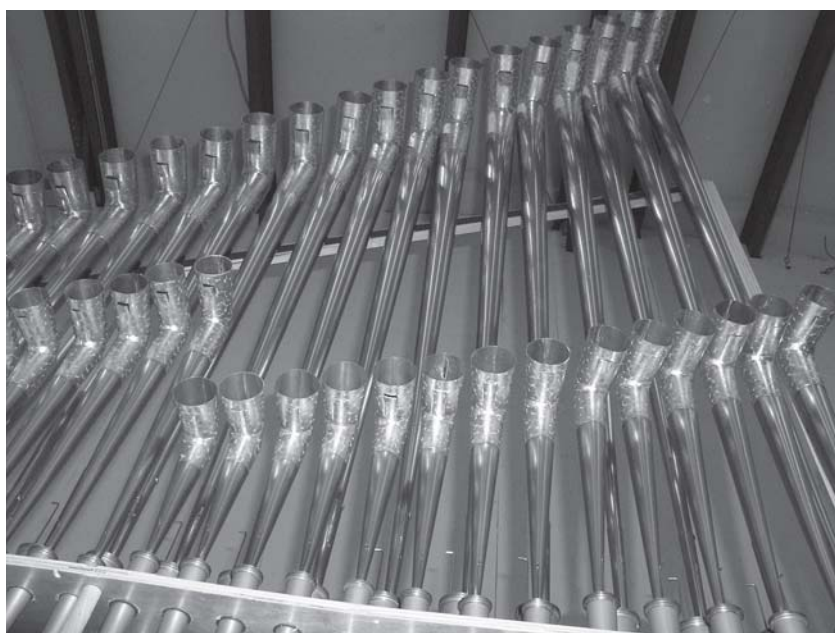
Fanfare Trumpet assembled in erecting room
