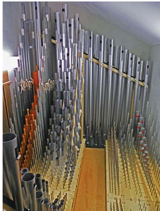
Panoramic view of the Swell division. In the background, mitered to follow the roof line, stands the 16' Bassoon, with the Pedal 16' Trombone behind. The angled ceiling and heavily braced walls enhance the tone's blend and clear projection into the sanctuary.
