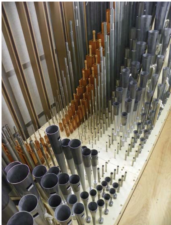
The Swell soundboard nearest the expression shutters (left to right): 8' Voile de Gambe, 8' Stopped Diapason, 8' Voix Céleste, 4' Principal, 8' Trumpet (with harmonic resonators), 8' Oboe d'Amore
