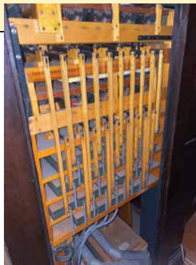
Mr. Skinner's stupendous vertical selector combination action (photo credit: John Bishop)
