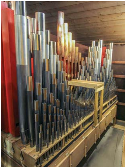
The 5-stop low-pressure section of the Great division (photo credit: Jonathan Ortloff)
