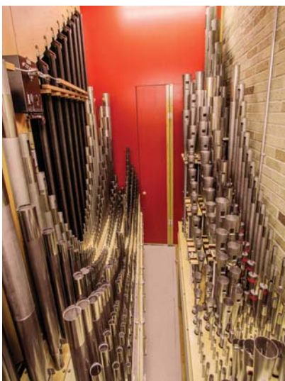
The 10-stop Swell division, with separate low and high-pressure sections (photo credit: Jonathan Ortloff)
