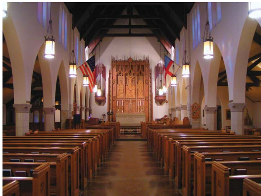
Long and tall geometric forms, with organ and choir located at the end of the long axis of the room, have excellent acoustical potential.
