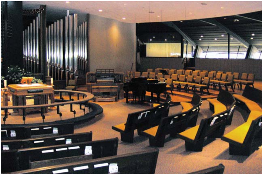
Concave and curved geometric forms, low ceilings, and limited air volumes typically cause acoustical difficulties.
