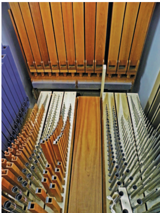
The compound Pedal/Great/Choir (left to right): Pedal 16' Sub Bass (painted Portland blue), 8' Bourdon , 8' Pedal/Choir Open Diapason , 4' Harmonic Flute , 8' Clarinet , 8' Vox Angelica , 8' Gemshorn , expression shutters. The 16' Bourdon extension stands in the background.
