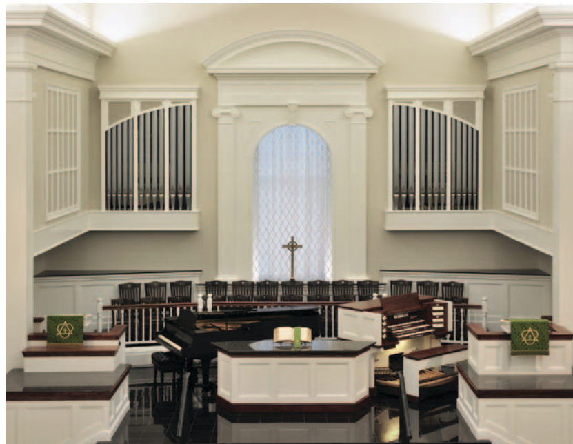
The new organ in the rebuilt chancel. The left chamber houses the Swell division and the Pedal 16' Trombone, with the right chamber accommodating the Choir, Great II, and Pedal flues. Behind the façades that flank the central window is the unenclosed Great I; the bottom octave of the division and the Haskelled Pedal 16' Contra Bass are behind the speaking façade on the left, and the main windchest is behind the non-speaking façade on the right.
