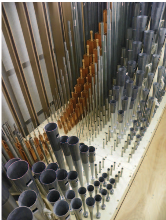
The Swell soundboard nearest the expression shutters (left to right): 8' Violo de Gambe , 8' Stopped Diapason , 8' Voix Céleste , 4' Principal , 8' Trumpet (with harmonic resonators), 8' Oboe d'Amore
