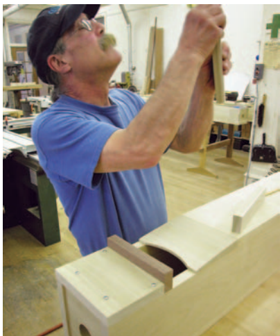
Constructing new wood pipes in the shop
