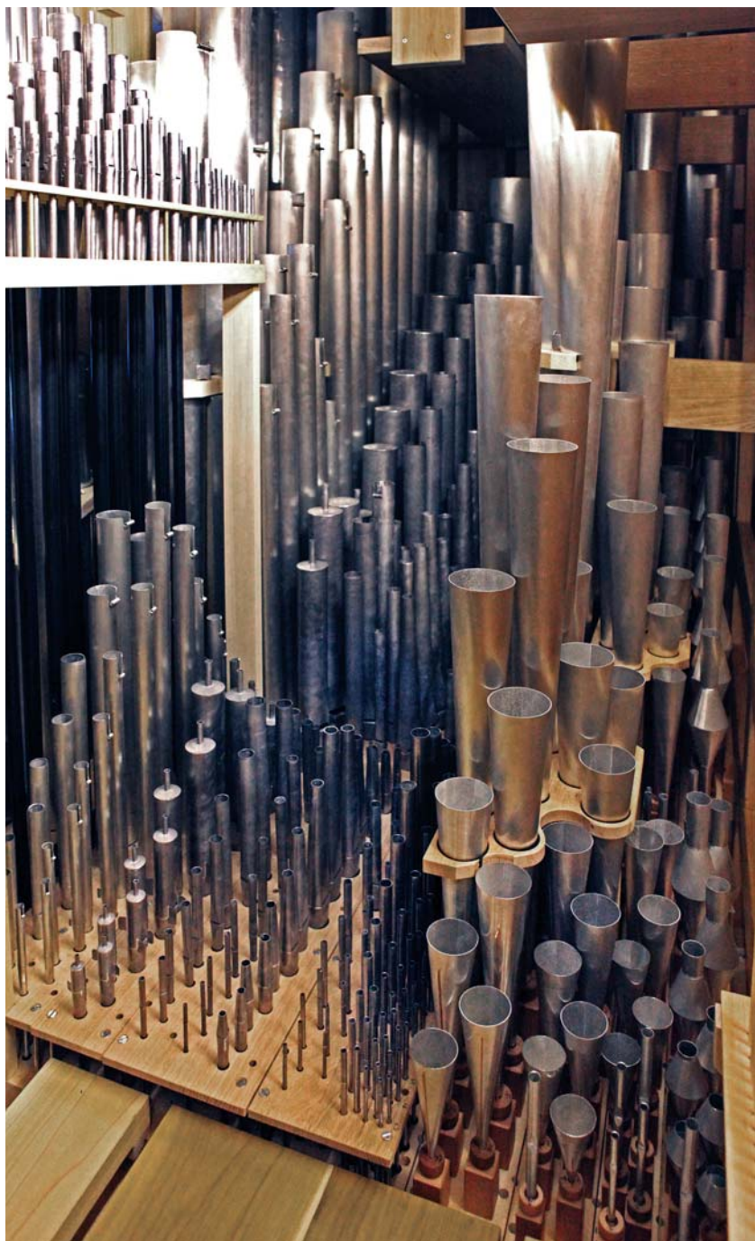
An inside look at the Great pipework, the "C" side of the organ. The tenor and treble sections are in major third arrangements, that is, neighboring pipes are a major third higher or lower, facilitating easier access (the walkboard is to the right, out of frame) and more efficient use of space. Top left is the mounted Cornet V.
