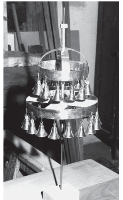
Photo 10. The “Chinese hat,” one of the elements of the “Turkish band.” This unit was manufactured by Fratelli Ruffatti as a copy in 1988 during the restoration of the Tronci organ, 1778, modified by Agati Tronci in 1898, in the church of S. Pietro at Casalguidi (Pistoia). The original had been removed and eliminated from the instrument during the 20th century.
