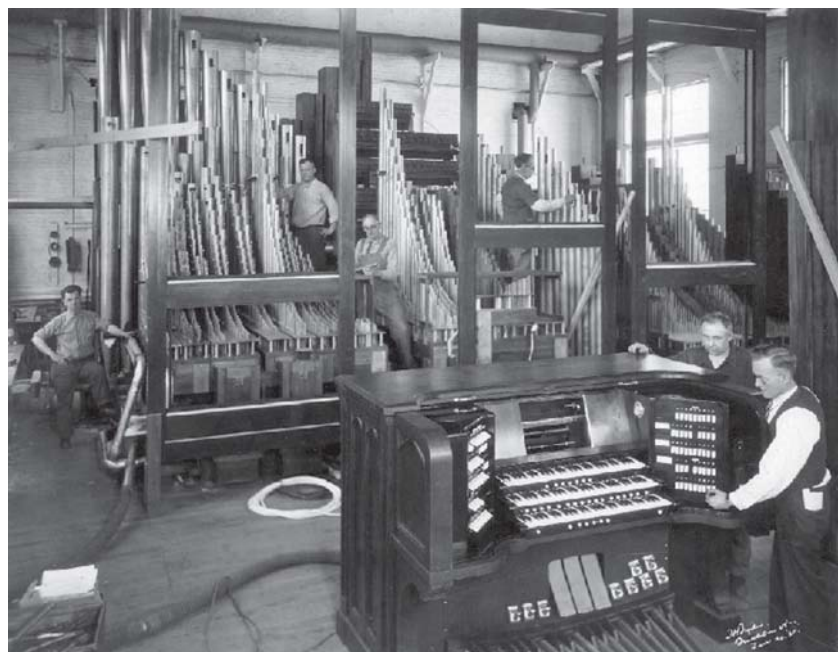
One of the identical organs for seven high schools in New York City, under construction in the Estey shop, Brattleboro, Vermont
