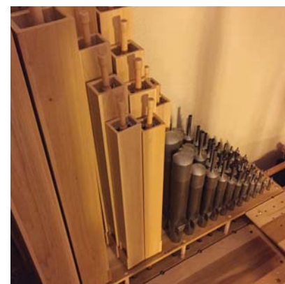
Rohrflute pipes installed
