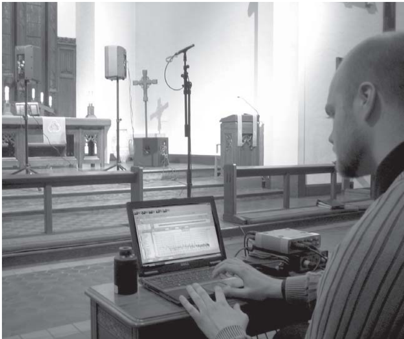
Eric Wolfram conducting acoustical testing with computer, microphones, speakers, and sound-generating equipment
