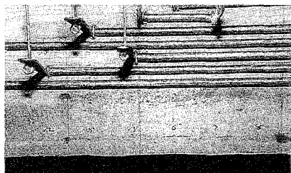
Callido's rollerboards were made of hand forged iron. The small elements placed under the rollers at their fastening point are made of lead. Callido applied them in order to reduce noise and friction.
