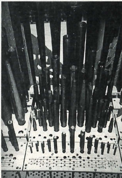
View of Great pipework before installation of mixture and reeds
